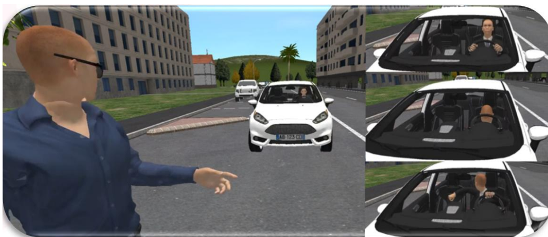
Figure 14 Example of driving scenarios implemented on the V-HCD platform to study interactions between a Pedestrian and CAV occupied by more or less attentive avatars
